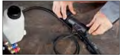
6. Lead out the flow control cable through the control cable outlet out of the housing.
