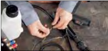
3. Connect the trigger cable to the flow control cable.
