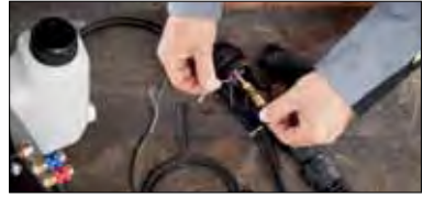
2. Disassemble end of the trigger cable.
