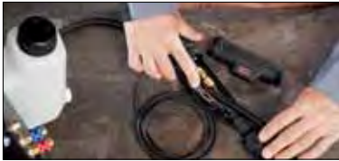
5. Insert the trigger and flow control cable into the connection housing.
