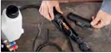
1. Open the machine side connection housing.
