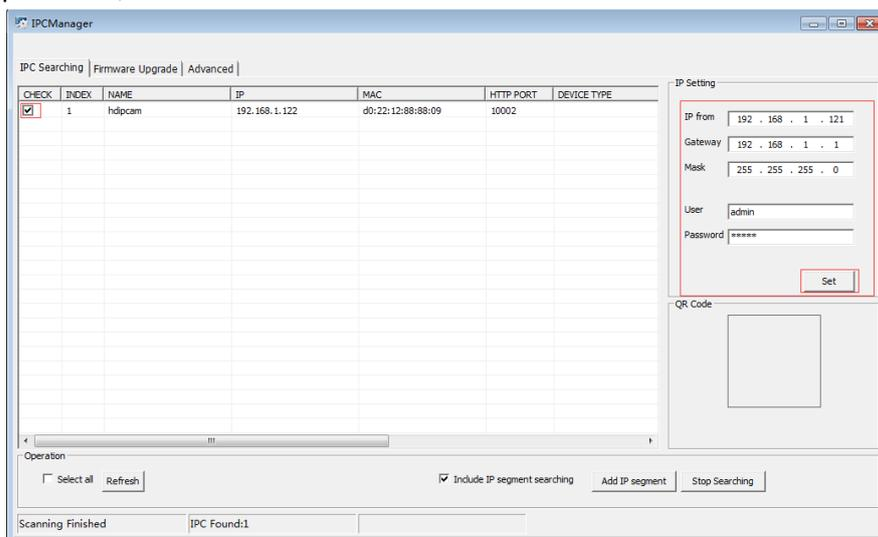
When there are many IP cameras in the list, select those you want to make changes, fill in the beginning IP address, gateway, mask, user name and password on the right part, and click "Set". Then IP addresses will be changed in sequence.
