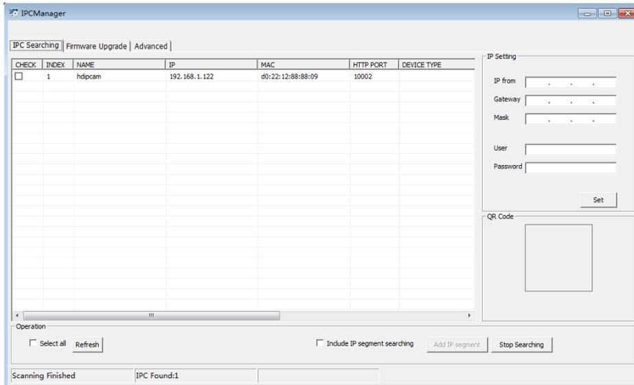
Quick search can be done for cameras in a certain IP segment. Click the checkbox of Include IP segment searching and click Add IP segment. On the new pop-up window, input beginning IP and ending IP, click Add, then a new IP segment will be added to the list.
