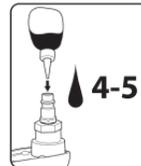
**NOTE:** Before the first use of the tool, apply 4-5 droplets of oil to the inlet opening before connecting the hose.
