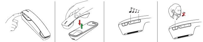
Jabra Handset 450 will always be powered on when docked in the handset cradle, and the cradle is plugged into a USB port. To turn off the Handset 450, press and hold (5 secs) the mute microphone button. Press the mute microphone button again, to turn back on. Lift the handset to answer a call. Put it back in the cradle to end it. Easy-controls allow you adjust volume and to mute calls.
