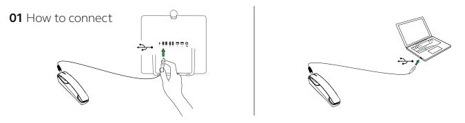
Jabra Handset 450's plug-and-play solution ensures that installation is truly hassle-free. Connect the USB cable to the handset cradle, and then plug the USB cable into any available USB port on your desk phone or your PC/Softphone. (Device dependent. See compatibility details)
