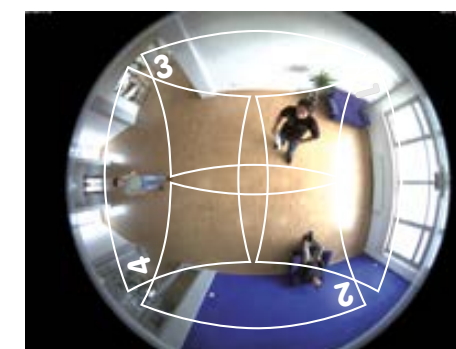
Four virtual PTZ cameras out of a single 360° hemispheric camera
