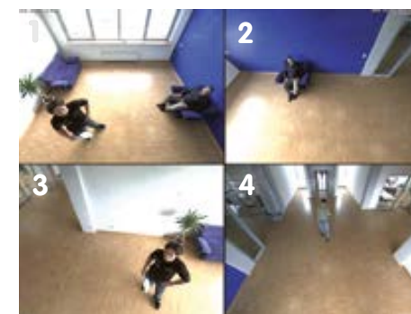
Four virtual PTZ cameras out of a single 360° hemispheric camera
