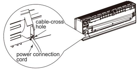
3. Remove the wire clip; connect the power connection cord to the wiring terminal according to the color; tighten the screw and then fix the power connection cord with wire clip.
