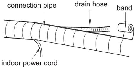
2. Reserve a certain length of drain hose and power cord for installation when binding them. When binding to a certain degree, separate the indoor power and then separate the drain hose.
