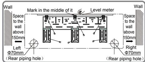
2. Open a piping hole with the diameter of  $\Phi 55$  or  $\Phi 70$  on the selected outlet pipe position. In order to drain smoothly, slant the piping hole on the wall slightly downward to the outdoor side with the gradient of 5-10°.
