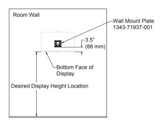
Drill the mounting holes for the wall mount plate as shown using the VESA 100 mm x 100 mm hole pattern. If needed, use the wall plate as a template for drilling the holes.
