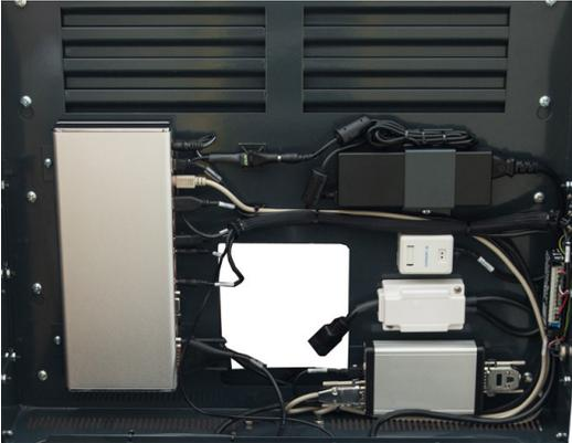
Connect the RJ45 network cable to the codec or connect a bare wire directly to the network junction block.
