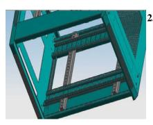
2.5: Installing the bayonet-type nut M6 on the mounting angle; and then using the allen screw M6x10 to connect the mounting profile and mounting angle;
