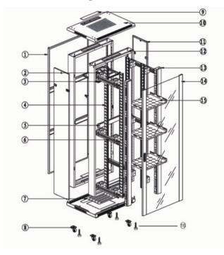
1、Assembling General Schematic Diagram (05A Series 600Width):
