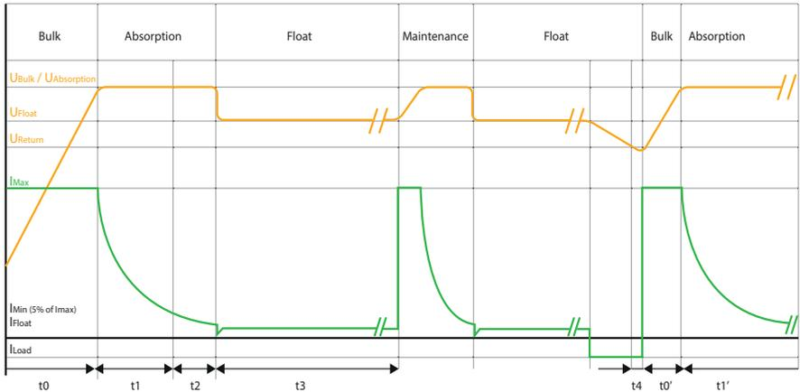
Figure 22. Charge curve
