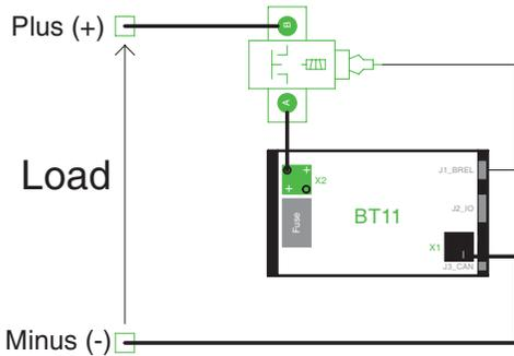
Figure 9. Connecting the battery to the load
