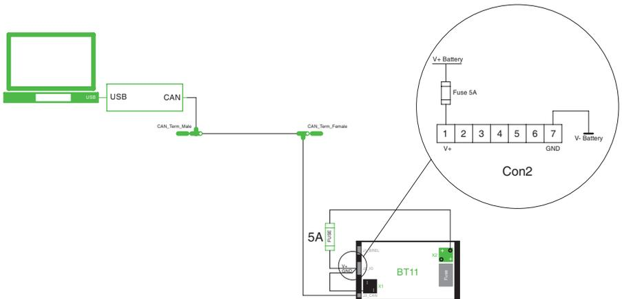
Figure 6. Use Con2 to power the CAN bus
