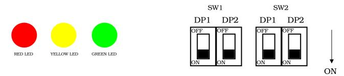
Only the set of dipswitch SW1 (the one on the left side) has effect on charging curve selection accordingly to the table above.
