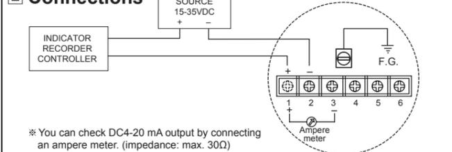
※ You can check DC4-20 mA output by connecting an ampere meter. (impedance: max. 30Ω)
