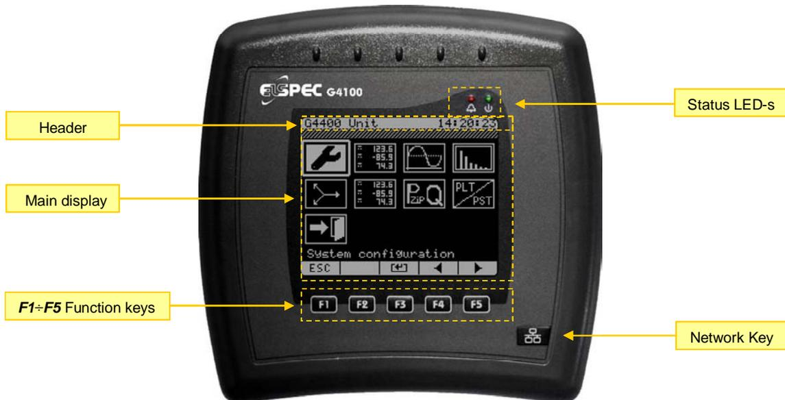
Figure 2: The Elspec G4100 Functional Display Unit
