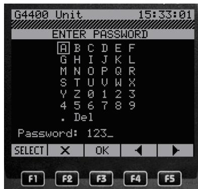
Delete the default user password, 123, by navigating to the "Del" key and pressing SELECT three times. Enter the password supplied by Elspec to authorize Admin level access by using the arrows to navigate to each character of the password and pressing SELECT. When the whole password is displayed on the screen, press OK. The previous configuration screen will appear, with "write" authorization.
