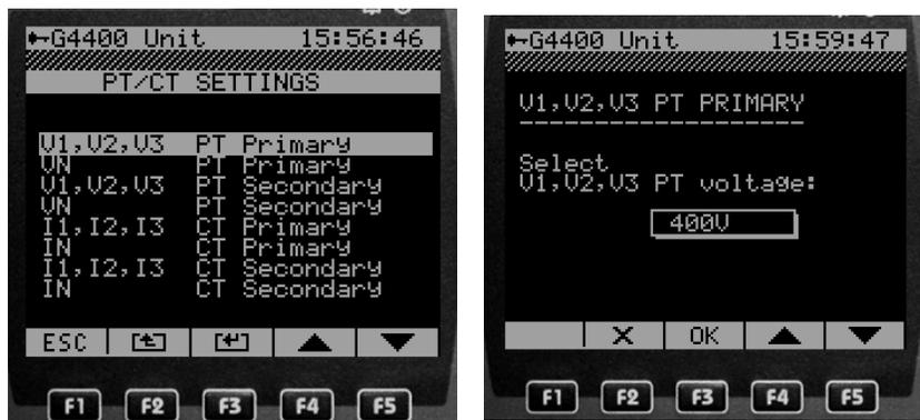
Figure 16:PT/CT Settings- inputting the Primary PT Value
