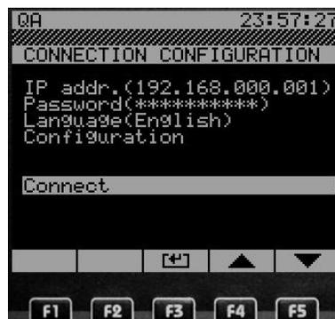
**F** Navigate to the IP address Field and press Enter. A list of previously visited G4400 instruments will appear:
