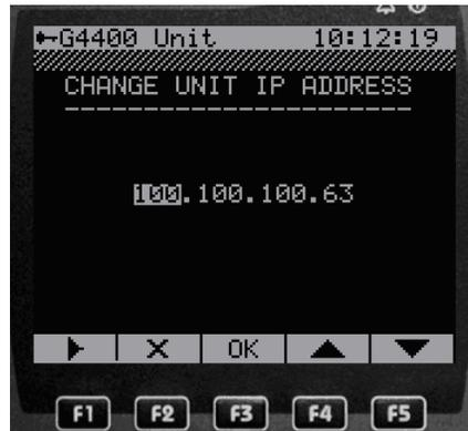
Navigate between the 4 address elements using the right arrow. Change the address elements using the up and down arrows. Lock in the address by pushing the OK button.
