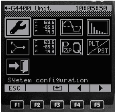
**F** Navigate to System configuration using right (▶) and left (◀) and then
