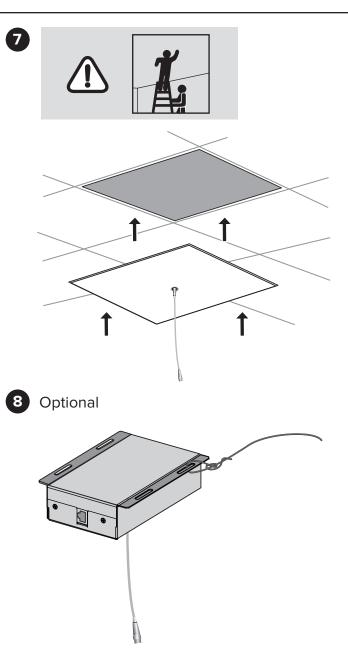
For added safety when removing the ceiling tile at a later time, securely attach the electronics enclosure to the ceiling supports using suitable wire or other hardware appropriate for your ceiling type and in accordance with local regulations. Be sure that the length of wire you use to secure the electronics enclosure is short enough to prevent the enclosure from striking the person removing the ceiling tile.
