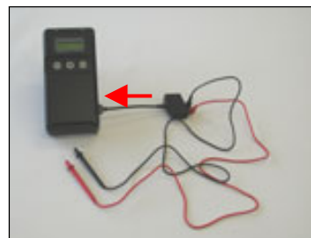
<Connecting the Measurement Adapter and Measurement Probe>
