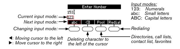
Press any key on the alphanumeric keypad or pick up handset to open the "Enter Number" screen. The current input mode is indicated in the information line underneath the cursor line. Press the left function key underneath the display to switch to the input mode indicated by the symbol directly above it in the function key line.
