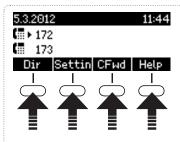
Press the function key to activate the function, open the list etc. depicted by the symbol above the key.
