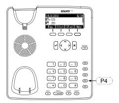
Press key P4 on the phone to show any ongoing activity on monitored extensions or lines on the display. For example: "153 157" indicates that extension 153 is calling extension 157; "153 157" (or "153 157") indicates that 153 is connected to 157 and that 153 is the caller, 157 the callee.
