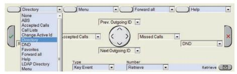
**Note:** These programmable key events are available when the phone is idle. You cannot change the functions that are available when there is activity on the phone. For example: When you are dialing, the available function keys are input mode selection, backspace, directory access, and redial.
