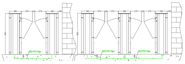
Figure 4-1B Single-Passage and Dual-Passage with FBL 5000
