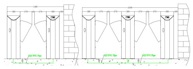
Figure 4-1A Single-Passage and Dual-Passage with FBL 4000
