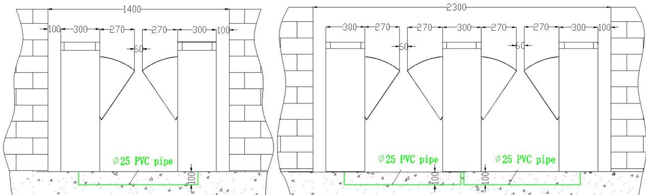
Figure 4-1A Single-Passage and Dual-Passage with FBL 1000
