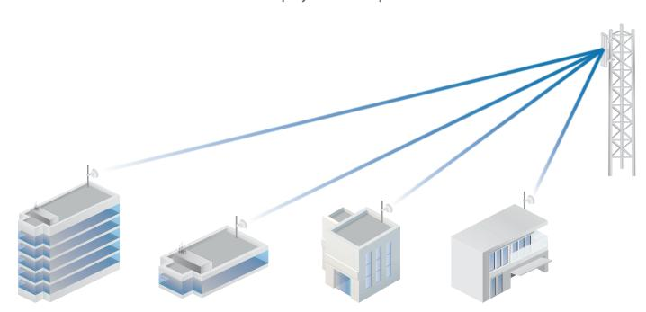
In a PtMP link, the LTU Pro functions as CPEs to the LTU Rocket, which is paired with an airMAX® sector antenna.
