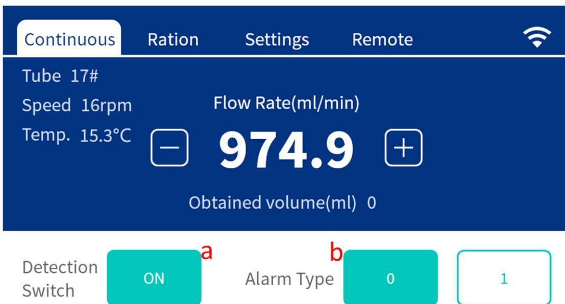
Figure 2-2-2-1 Continuous mode liquid level detection setting
