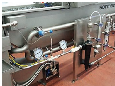
G3 wall-mount requires minimal space (left); Typical injector arrangement and degas configuration.
