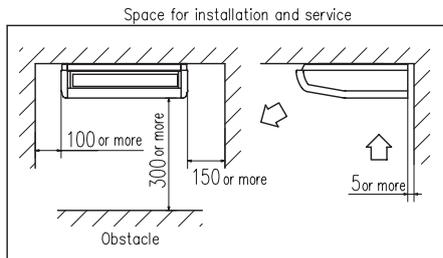
Make a space of [ f ] or more between the units when installing more than one.
