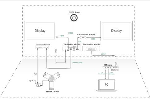
**Note:** For more information about the installation and deployment of accessories (for example, the installation of mini-PC or UVC30 camera), refer to the Quick Start Guide of the corresponding accessory.
