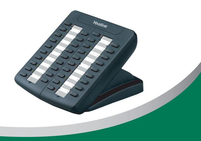
Yealink EXP38 Expansion Module is designed for improving the power and flexibility of Yealink advanced IP phones SIP-T28P & SIP-T26P. It features 38 fully programmable DSS keys each with a dual-color LED, connected to and controlled by the IP Phone with an RJ-12 cable line. It creates up to 228 additional programmable extensions when 6 EXP38 are daisy chained with the IP Phone.
