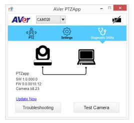
e. Test Camera: Click the "Test Camera" to check the camera video display status. You can adjust the camera direction and view of the zoom in/out. To leave the page, click the Abort Diagnostic button.
