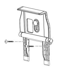
Connect to USB cable and then secure the clip knob firmly to prevent from falling off
