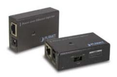
Using the Planet POE adapters, you can power most DC network devices (hubs, Wireless access points, cameras etc) over the same Cat 5/5e cable used to connect the device to the network.
