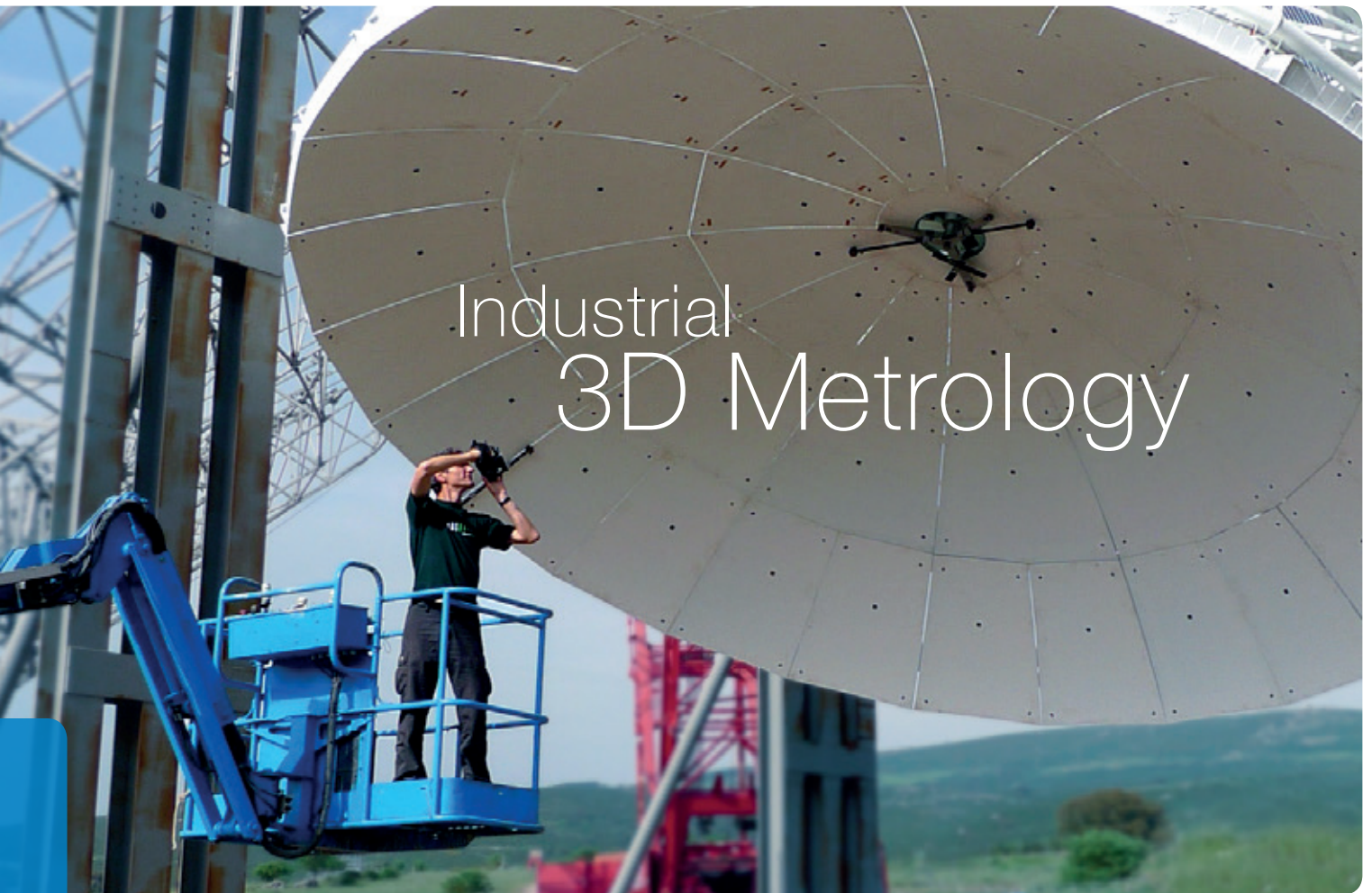
Measurement of a satellite antenna with DPA (photo: sigma3d GmbH)
