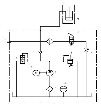
Gear Pump 2. Motor 3. Filter 4. Check-Valve
