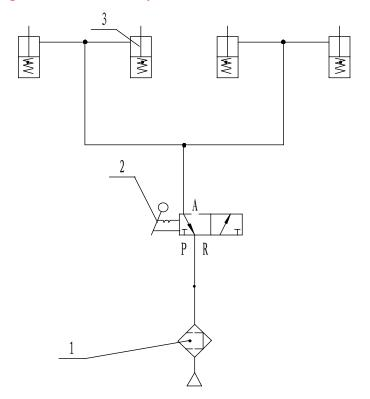
1. Air Source 2. Air Control Valve 3. Air Cylinder
