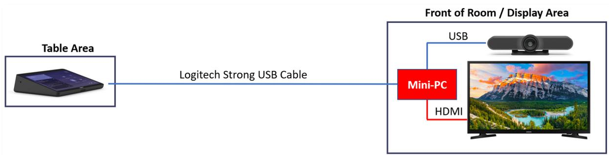
Figure 4: Logitech Small Rooms Solution – Installation Diagram – Includes Logitech Tap and MeetUp
