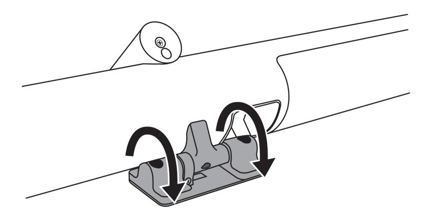
Screw the PanaCast 50 to the table stand using the supplied M5x12 screws and a 4mm hex key.
