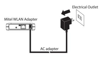
While reconnecting the AC plug to the outlet, press and hold the push switch at the front of the Mitel WLAN Adapter. Keep pressing and the factory default configuration will begin.
