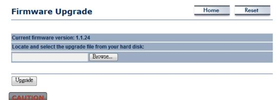
The upgrade process may take few minutes. Please do not power off the device as this may cause the device to crash or become unusable. The ENH202 will restart automatically once the upgrade is complete.
