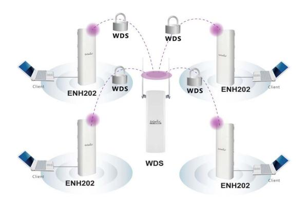
WDS Bridge Mode is unlike Access Point Mode. APs linked by WDS are using the same wireless channel, and connecting excessive numbers of APs on the same channel may result in lower throughput. Please be aware to avoid loop connections; otherwise enable the Spanning Tree Function.
