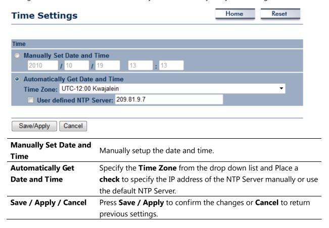
Pressing Save / Apply will change the settings immediately. It is not reversible unless the settings are changed again or the device is reset.
