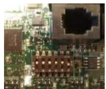
Figure 6 DIP switch positions for using a heater
