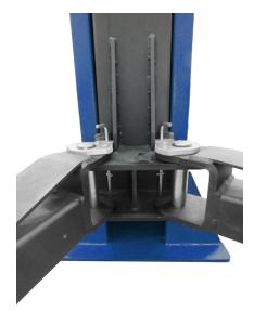
Automatic locking & unlocking of arms during on floor
