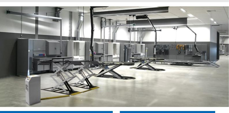
THE CDS 35 DOUBLE SCISSOR LIFT HAS A PROFILE TO DRIVE/ROLL ANY VEHICLE OVER IT FOR FAST REPAIR WORK.
