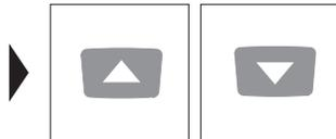
Press the “▲” key to increase the output power. The measurement range is from -2 dBm to -8 dBm. Each time you press it , the value increases by 0.1 dBm.
