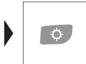
Press the backlighting Key to switch the backlighting of the LCD on and off.
