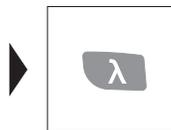
Press the "λ" Key to switch the wavelength between 1310nm, 1550nm for FHS2D02, 850nm, 1300nm for FHS2D03, 1310nm, 1490nm and 1550nm for FHS2T01.
