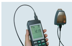
Inspection of transmitters with 4 to 20 mA interface
