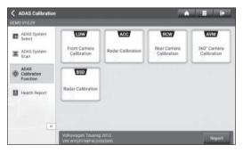
Tap the desired calibration item (Take **Front Camera Calibration** for example), the following screen will appear:
