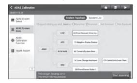
The ADAS systems can be displayed in form of topology or list. Tap **Start Scanning** to start reading DTCs. After scanning is complete, tap the system displayed in red to view the existing DTCs, or tap the system functioning normally to perform other diagnostic functions. For details on diagnostic function, see Chapter 6.2.3.
