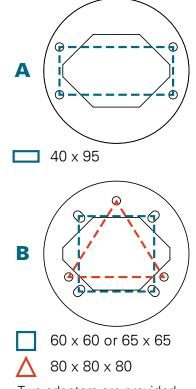
Two adapters are provided. Stick the appropriate one on top of the box, to blind open holes if necessary.
