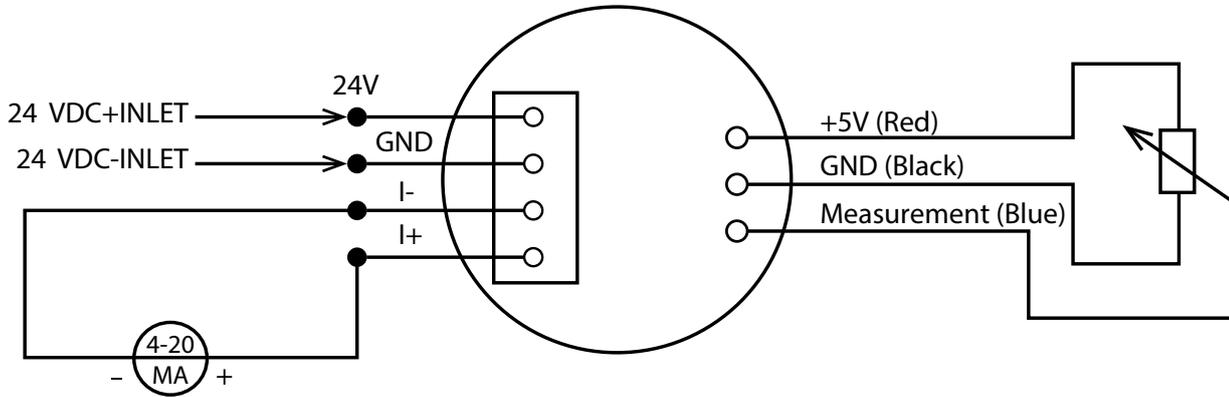
You can connect + end from transformer to 24V and - end from transformer to GND(Ground) then I- end to our system mA- end, I+ end to our system mA+ end. After that connections, systems will be ready. With this signal, you can start / stop the pump, open / close the valve or get the alarm signal via your automation system.
