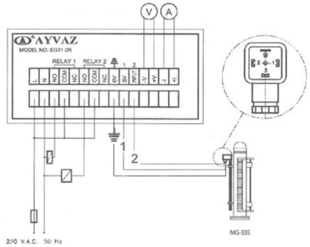
As shown in the above drawing, the system can be activated by connecting the grounding terminal to 0V, 1 terminal to 5V, 2 terminals to INPUT, 0-10V or 4-20mA automation output can be taken over the panel.
