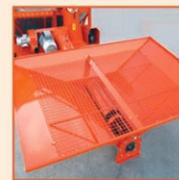
Loading hopper 2400 × 1500 mm for PRT200-250
