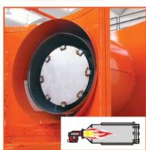
Combustion chamber (direct flame)
