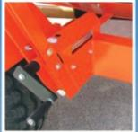
Adjustment of auger grain flow
