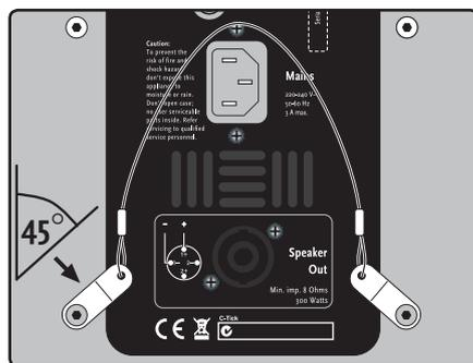
**Attaching the curving cable:** The curving cable lets you precisely aim the flown PR:O 8 A cab. It attaches to the back of the PR:O 8 A.
