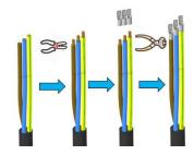
**Note:** Ensure that the insulation rubber of the AC input cable is flush with the indicator position on the bottom plate.
