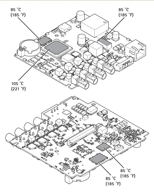
Maximum allowable temperatures. If the ambient temperature is 35  $^{\circ}$ C (95  $^{\circ}$ F) or higher, the temperature of the components increases and they must be cooled.
