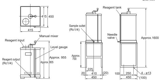
• Reagent mixing tank with mobile stand (RC401G-C)
