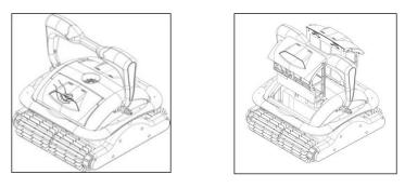
2. Push the buckles towards the middle and move the filter panel outwards
