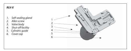
The valve assembly features valve body and a self-sealing gland pre-mounted with 2 O-rings - one for sealing against the radiator and one for sealing in the valve housing.
