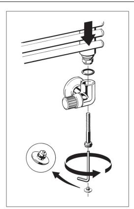
The self-sealing gland is mounting in radiator inlet and outlet using a 17 mm hexagonal key.
