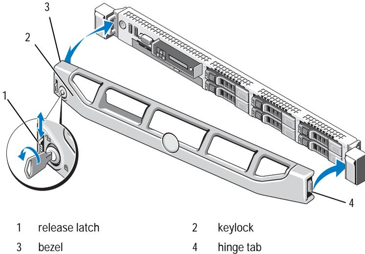
To replace the optional bezel, hook the right end of the bezel onto the chassis, then fit the free end of the bezel onto the system. Secure the bezel with the keylock. See Figure 3-2.
