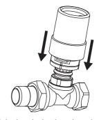
2. Install the hand wheel on the valve along with the guide slots.
