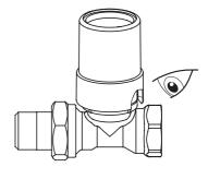
4. Visually check that the bottom is aligned with the indicator line.
