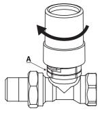
3. Turn the hand wheel clockwise until the bottom reaches the indicator line (A).
