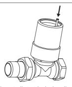
5. Place the spindle inside the handle.
